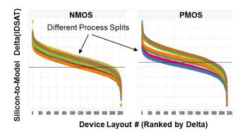
Fig. 4. Distribution of measured device performance (IDSAT) with respect to their model values for more than 2200 device layouts, NMOS and PMOS transistors. Direct Probe CV was used to collect the data from several wafers processed with different gate process conditions
