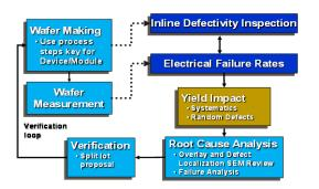
Fig. 2. Short Flow characterization loop using electrically testable structures on CV wafers.
