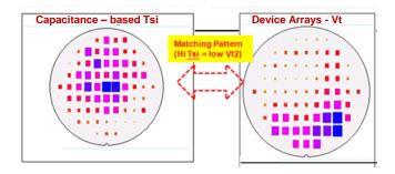
Fig. 3. Wafer level uniformity of Silicon Thickness extracted from Capacitance measurements and Vt variability in Transistor Arrays
