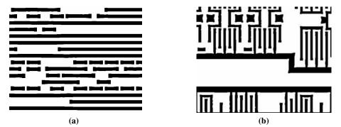
Figure 4: Metal layer model-based OPC (a) pdBRIX (b) Standard Cells
