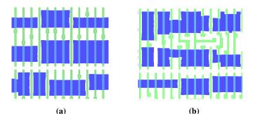
Figure 3: Active layer model-based OPC (a) pdBRIX (b) Standard Cells
