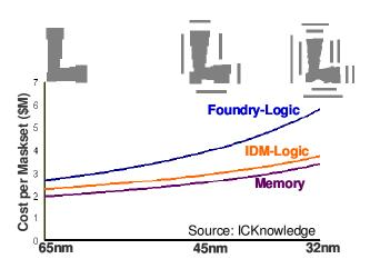
Figure 1: Increasing OPC complexity and mask costs
