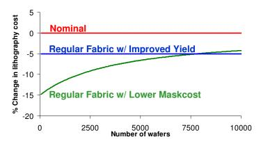
Figure 6: Implications on lithography cost per layer by improving yield or reducing mask costs as a function product volume
