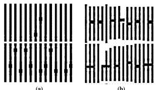
Figure 2: Poly layer model-based OPC (a) pdBRIX (b) Standard Cells
