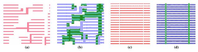
Figure 7: 32nm Poly (a) Standard cell design (b) Standard Cell OPC (c) pdBRIX design (d) pdBRIX OPC
